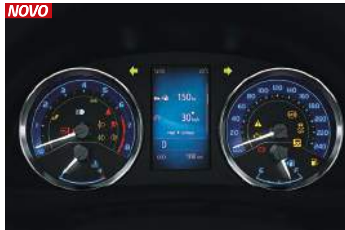
Painel com tela central de TFT digital e colorido*
